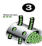
The flow of natural gas from the opened fissures is increased.
